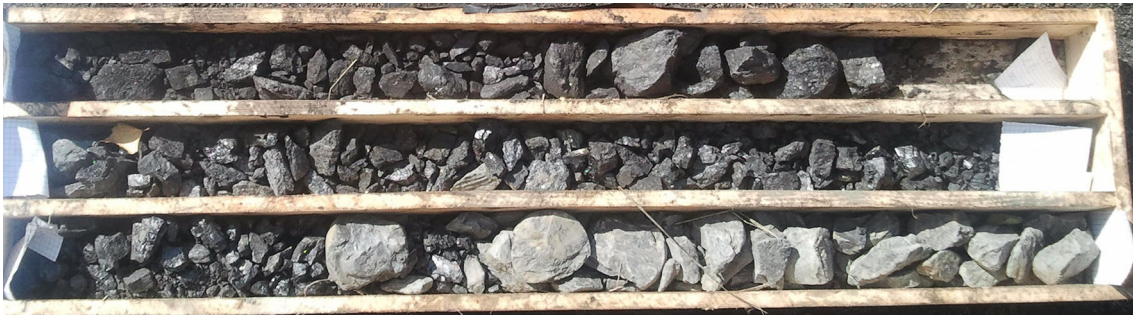
Fig. 2 Entirely crushed core from the floor of the work site
