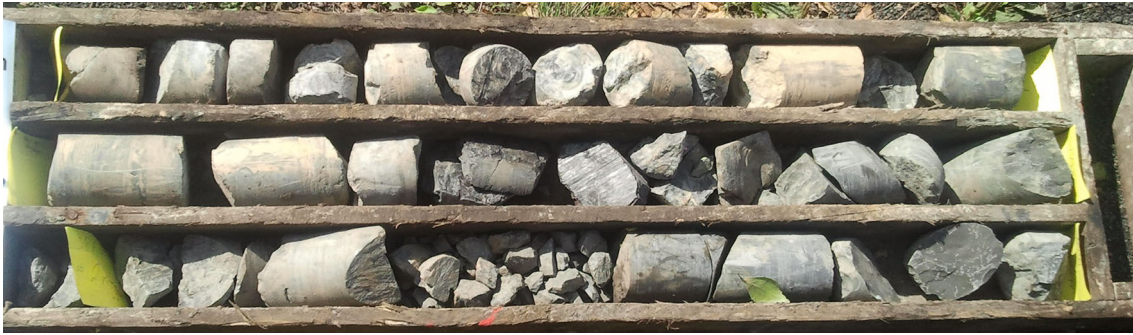
Fig. 1 Intensely crushed core from the floor of the work site
