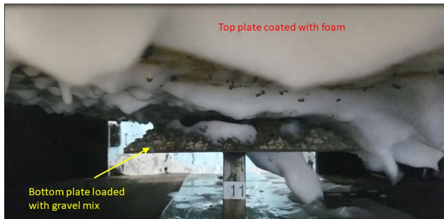
**Fig. 3** Inside view of the test chamber (shown in Fig. 1) as the bottom plate completes a traverse. It is at location *Plate drops/lowers halfway* as stated in Table 2
