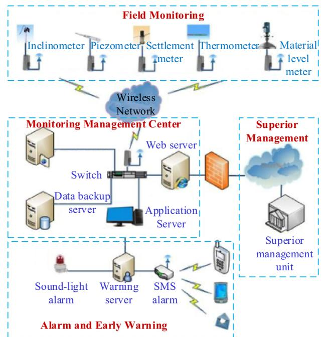
**Fig. 2** Structure of real-time monitoring system for CB deformation
