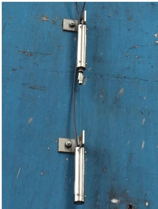
**Fig. 4** Installation of biaxial inclinometers
