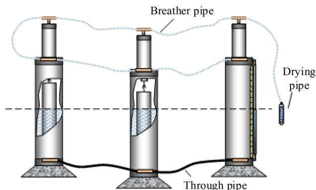
**Fig. 5** Schematic of components of hydrostatic leveling system
