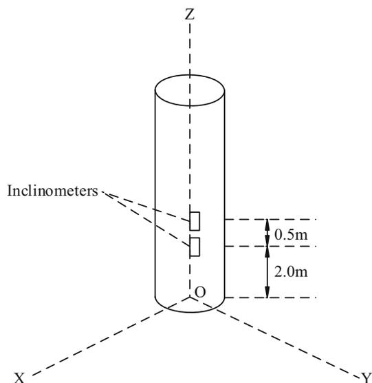
**Fig. 3** Installation positions of biaxial inclinometers
