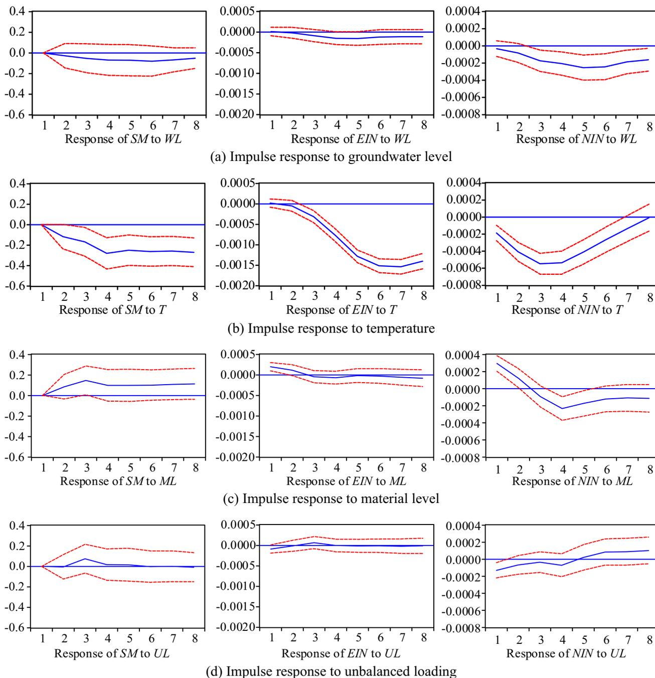
**Fig. 10** Impulse response of CB deformation to each influencing factor
