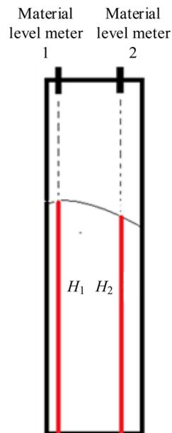
**Fig. 8** Schematic of monitoring of material level
