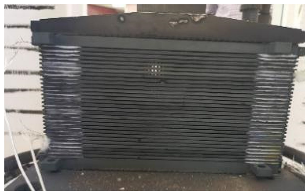
Fig. 8 Image of the kW-level stack for SOFC/SOEC applications
