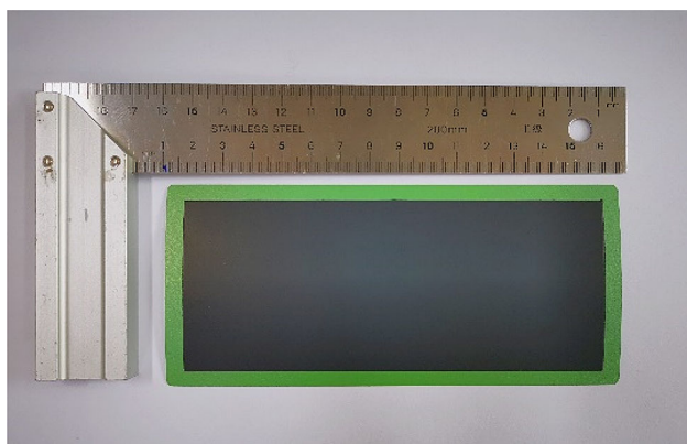
Fig. 7 Anode-supported SOFC/SOEC single cell
