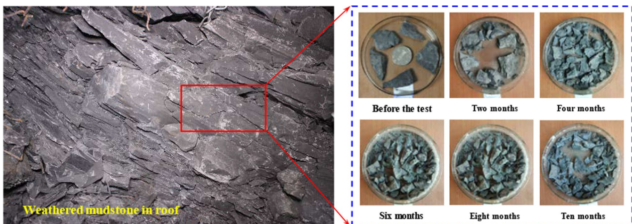
Fig. 9 Test results for a dry–wet cycle of immersed mudstone
