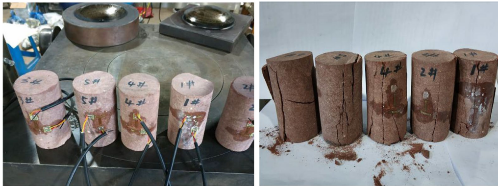
Fig. 5 Standard rock sample and the broken sample after test
