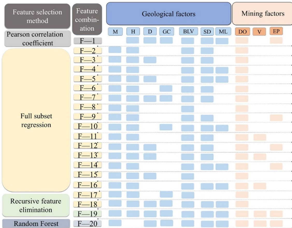
Fig. 4 Combination set of feature parameters affecting gas emission. Notes: F-1 represents the first feature combination, F-2 represents the second feature combination, and so on. The feature combination of the same color is selected by the corresponding feature selection method on the left
