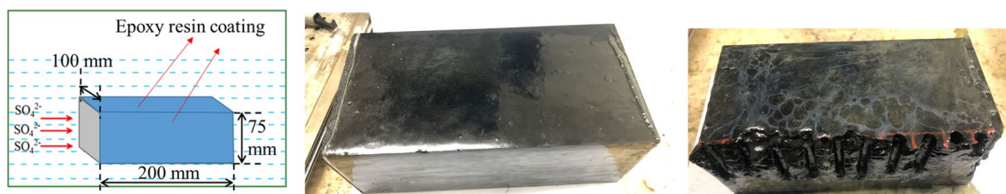
Fig. 2 Coal sample preparation and coring
