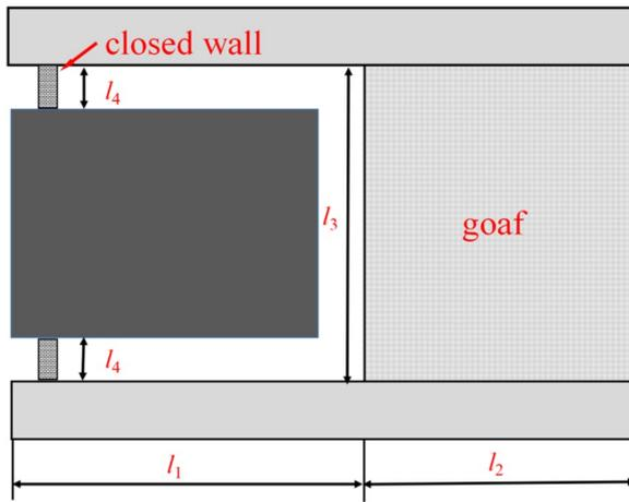
Fig. 2 Schematic diagram of closed area of mine
