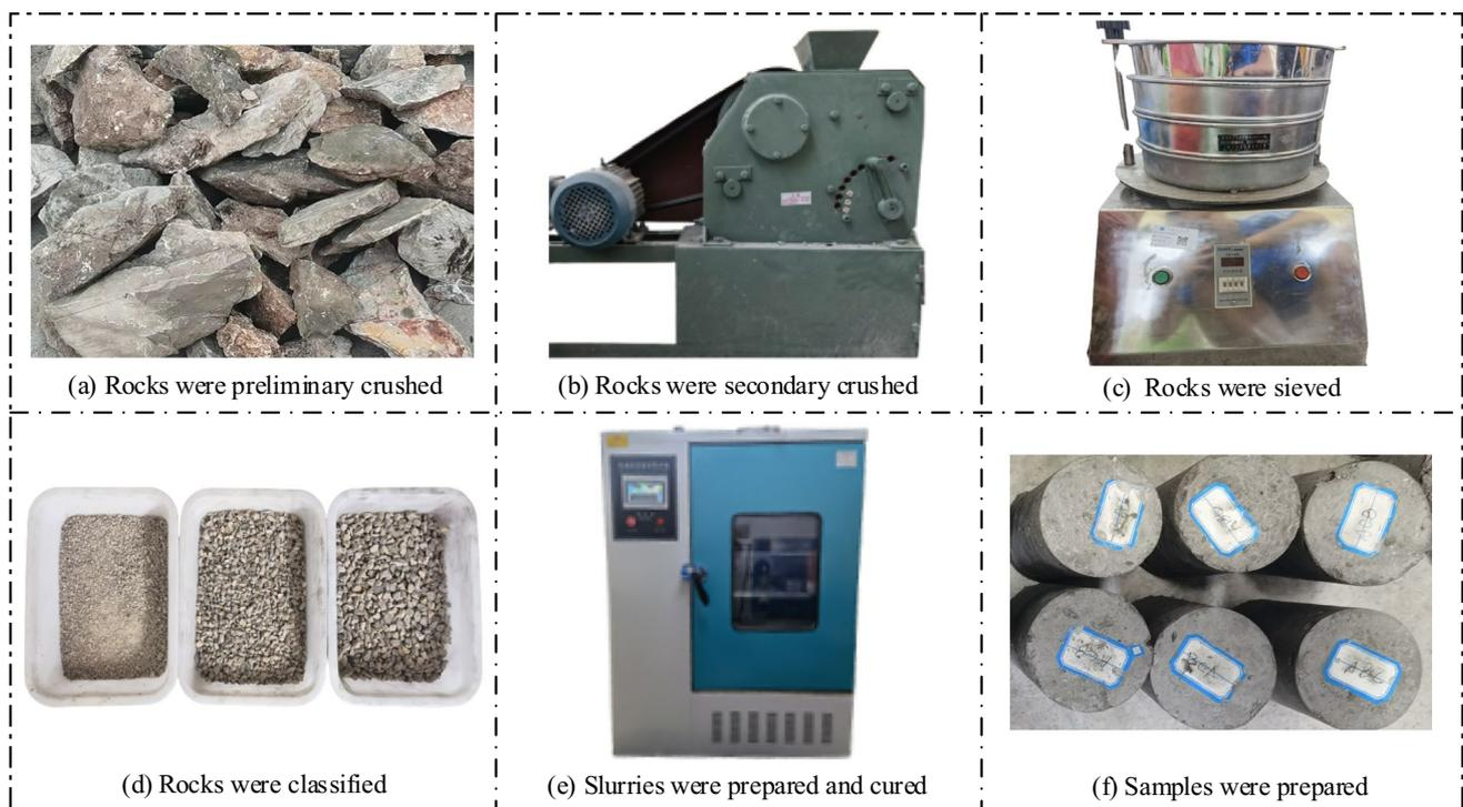
**Fig. 1** Preparation process for similar materials of weakly cemented fault rocks
