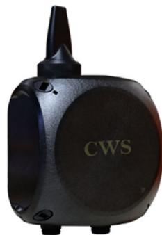
SmartConnect mesh networking protocol (Bhattacharya et al. 2013). The CWS consists of a radio module, a sensor module and a power module. The radio module manages the wireless communication, the sensor module manages the hardware interface for operating the sprinkler valves and the power module manages the power for the CWS and the motorized valves connected to the sprinklers.
