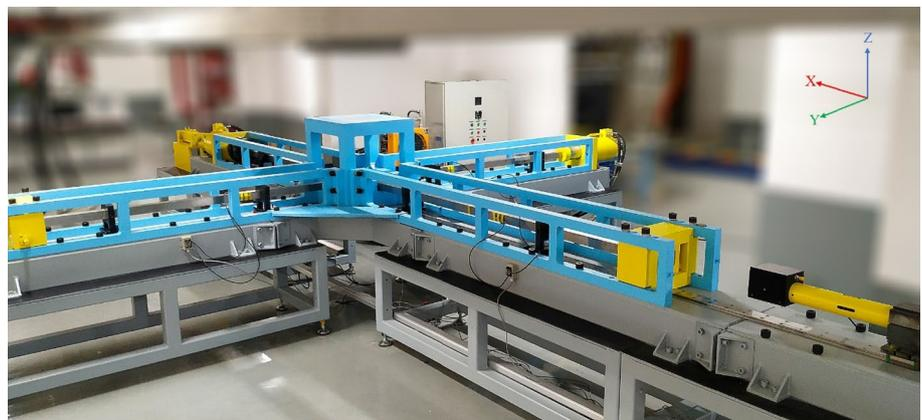
$A_s$  and  $L$  represent the initial cross-sectional area and length of the sample, respectively;  $\epsilon_{in}(t)$ ,  $\epsilon_{re}(t)$ , and  $\epsilon_{tr}(t)$  denote the incident strain, reflected strain, and transmitted strain in the  $X$ -direction, respectively;  $\epsilon_{y1}(t)$  and  $\epsilon_{y2}(t)$  are the strains in the two output rods in the  $Y$ -direction.
