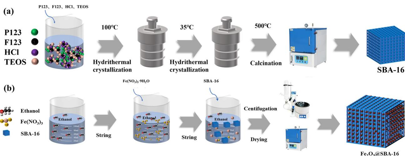
Fig. 2 a Preparation process of SBA-16 b Preparation process of  $\text{Fe}_2\text{O}_3@\text{SBA-16}$
