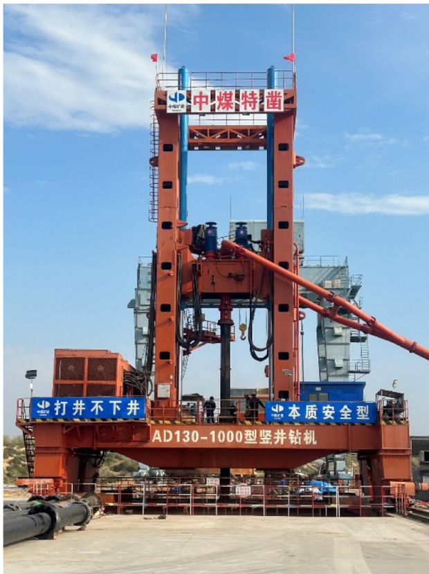
Fig. 1 AD130/1000 shaft drilling rig
