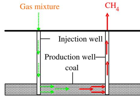
**Fig. 3** Schematic diagram of G-ECBM technology (After Fang and Li 2013b)
