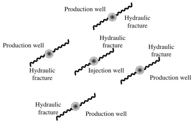
**Fig. 2** 5-spot pattern configuration of the hydraulic fracturing wells for ECBM operation
