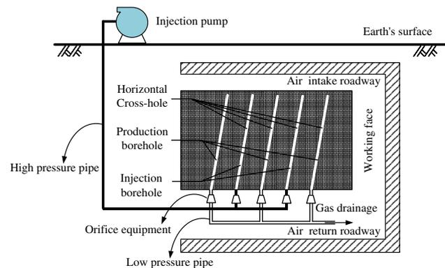
**Fig. 4** Typical layout for an underground ECBM system (Fang and Li 2013b)
