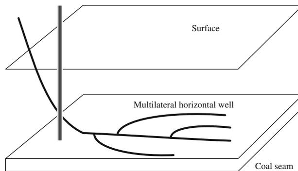
**Fig. 1** Layout of well pattern of multilateral horizontal well for ECBM operation (After Pan 2012)
