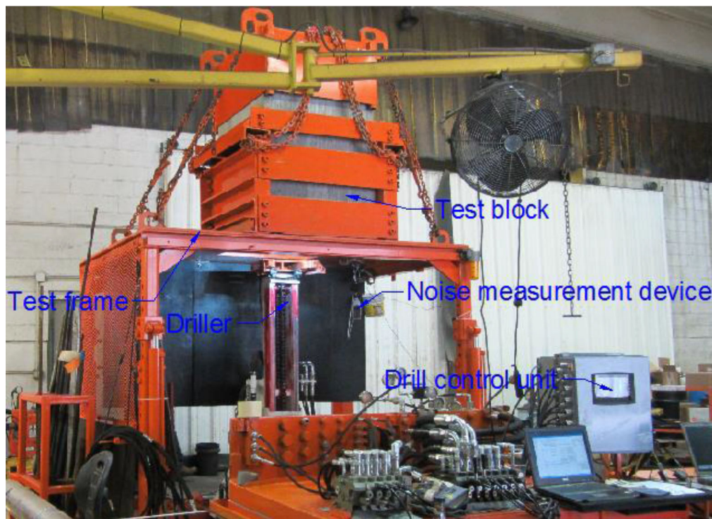
Fig. 3 Experimental setup of the drilling dust study
