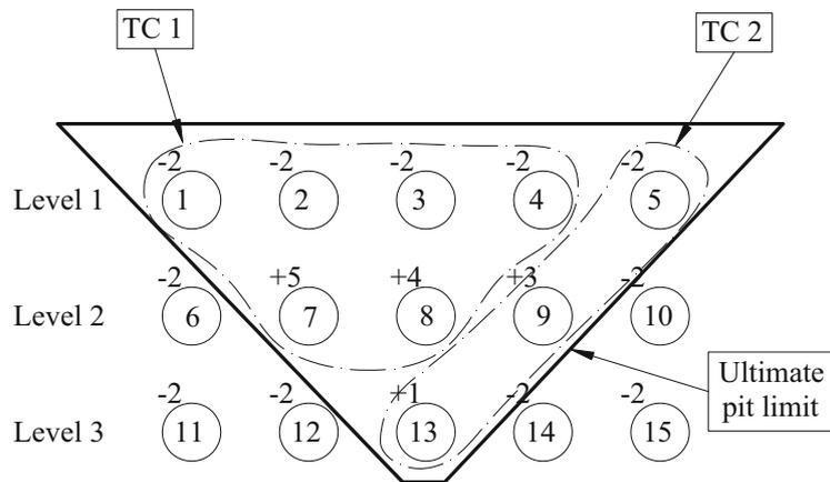
Fig. 6 Two TopCones were generated with minimum size of three blocks
