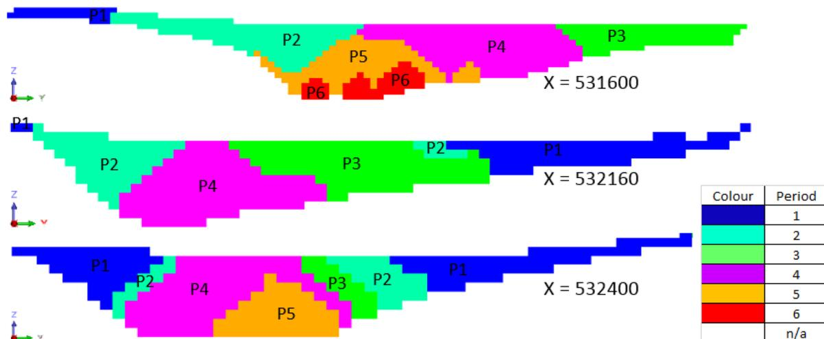
**Fig. 8** Typical cross-sections of mining sequence generated by TCA-based IP model
