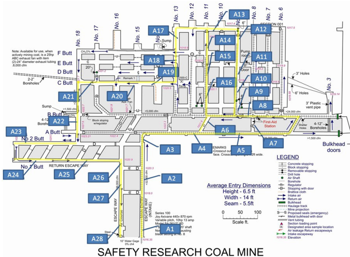
Fig. 1 SRCM layout and airflow measuring stations
