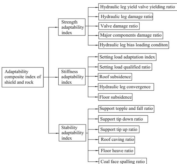
**Fig. 3** Hydraulic support and surrounding rock adaptability evaluation indexes
