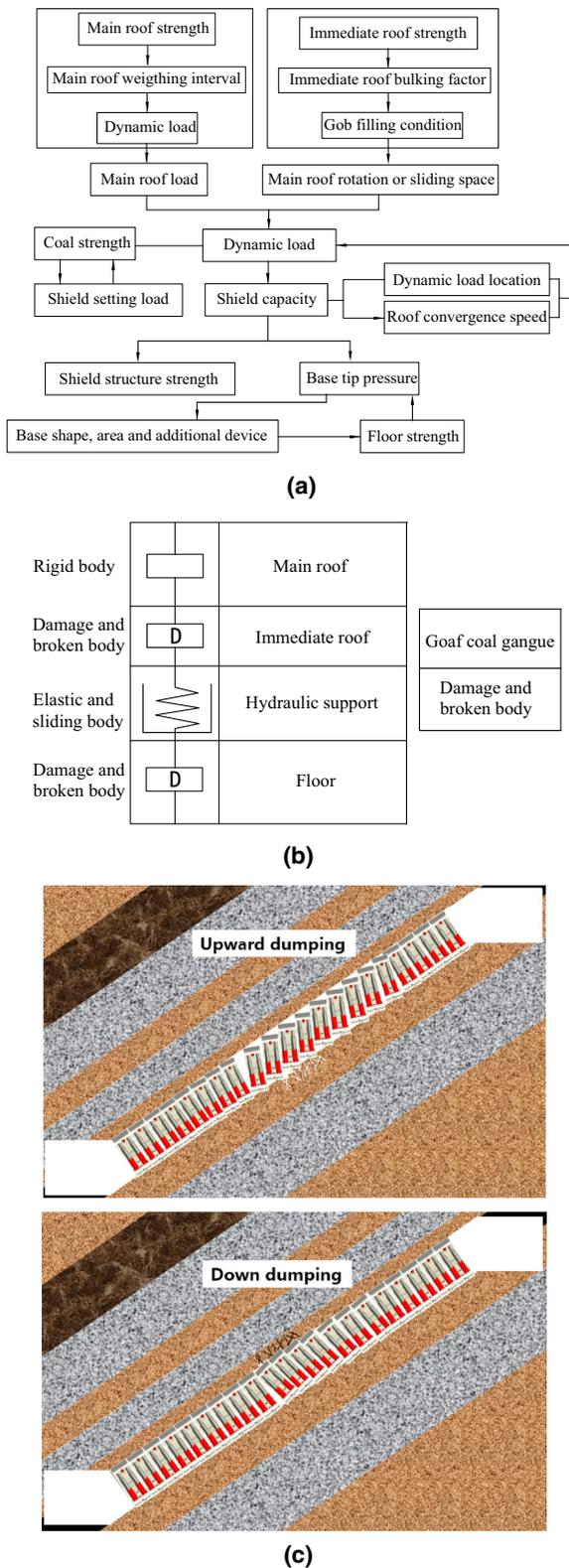
**Fig. 1** Coupling relationship between hydraulic support and surrounding rock. **a** Strength coupling relationship, **b** Stiffness coupling relationship, **c** Stability coupling relationship
