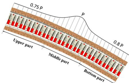
**Fig. 10** Mining ground pressure distribution characteristics in steep dipping face
