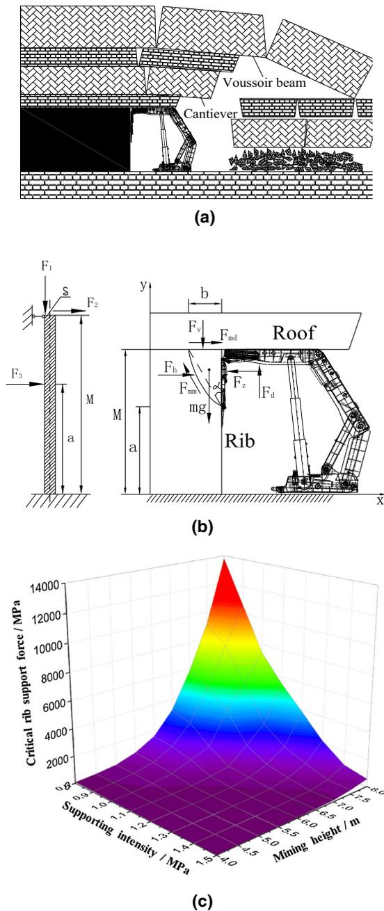
**Fig. 4** Coupling mechanical model between hydraulic support and surrounding rock. **a** “Cantilever + voussoir beam” structural mechanics model, **b** “Tension-slippage” mechanical model, **c** relationship of supporting intensity and critical rib support force in different mining height
