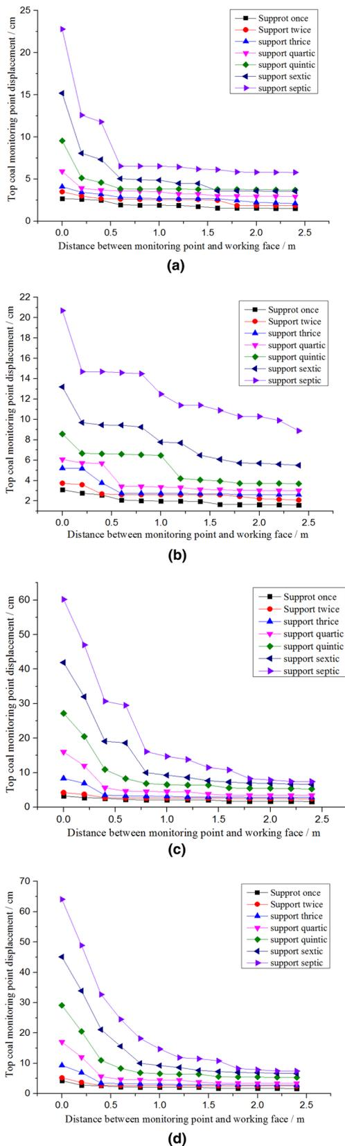
◀Fig. 6 Top-coal time-displacement curve due to hydraulic support supporting again and again to top-coal. **a** Supporting stress 0.3 MPa, **b** Supporting stress 0.6 MPa, **c** Supporting stress 0.9 MPa, **d** supporting stress 1.2 MPa
