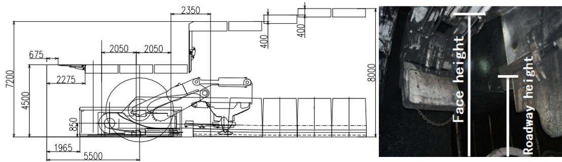
**Fig. 5** Equipment matching manner for super cutting height working face
