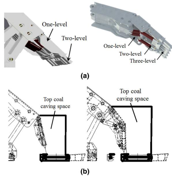
Fig. 7 Two types of top coal caving. **a** Top coal caving device contrast, **b** Top coal caving space contrast
