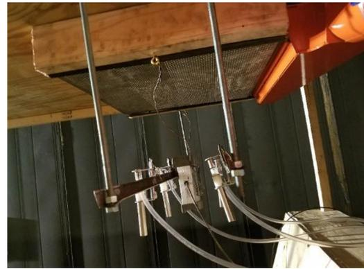
**Fig. 6** Photo showing the sampling locations, both the pDR-1000 and 4 gravimetric samplers, underneath the CAC
