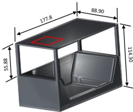
**Fig. 1** The center-drive shuttle car cab for the Joy 10SC32AA (dimensions in centimeters). The red outline shows the location of the canopy air curtain underneath the cab roof during testing (drawing by NIOSH)
