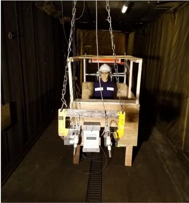
**Fig. 4** Photo showing the setup of the center-drive cab for testing with the manikin used for centering the CAC over the shuttle car operator
