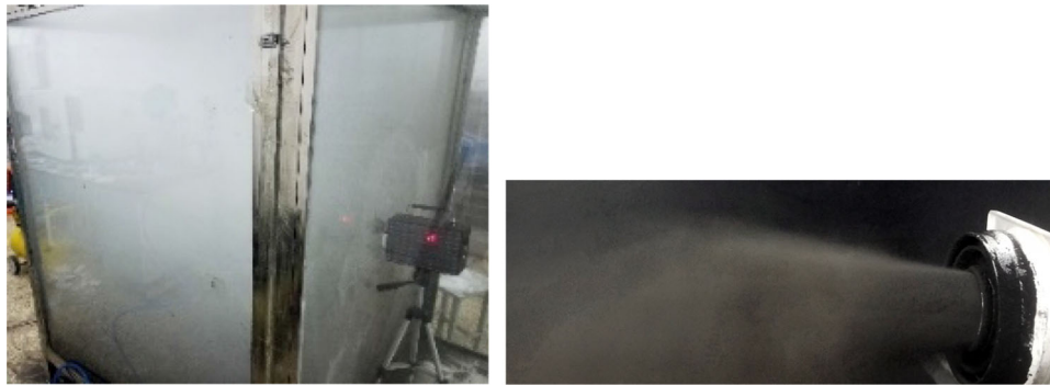
Fig. 17 Dust control experiment (left) dust sampler sampling and atomizing, (right) coal dust emission
