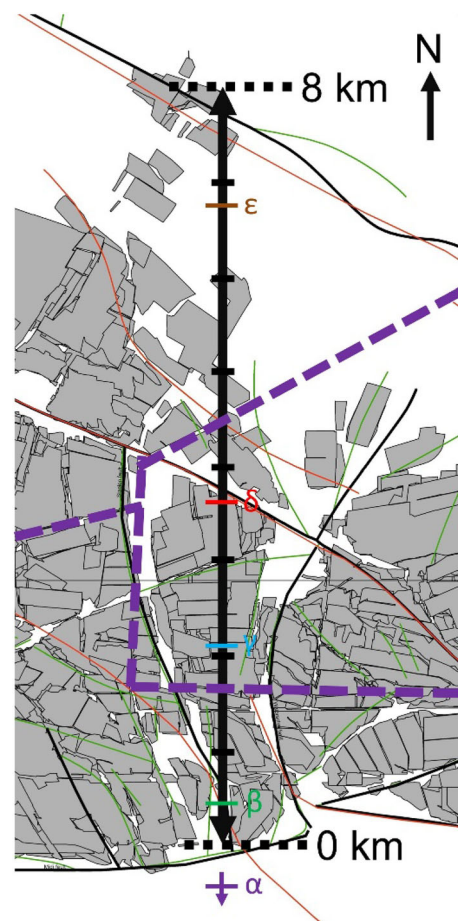
Fig. 6 Map of the mined panels below and around the central transect line, indicated by the black double arrow. The total north–south distance of the mined area is 8 km. The average positions of the five locations are presented along the central line (same colour code as Fig. 8; location \alpha is situated at a distance of -3.125 km). Concession lines between the three coal mines are indicated in purple (south and west: Winterslag mine; middle: Waterschei mine; north: Zwartberg mine)
