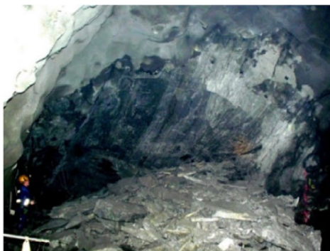
(a) A self-initiated strain burst occurred in a hard quartzite mine with 1000 m of mining depth
