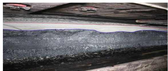
Fig. 8 Coal and rock boundary of 1.1-m thin coal seam working face
