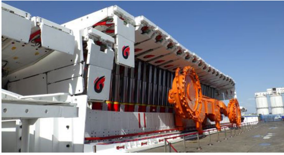
Fig. 11 Complete set of fully mechanized mining equipment for super-large mining heights
