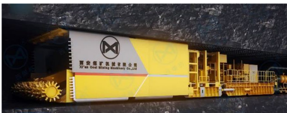
Fig. 12 Shield-type intelligent tunneling robot system
