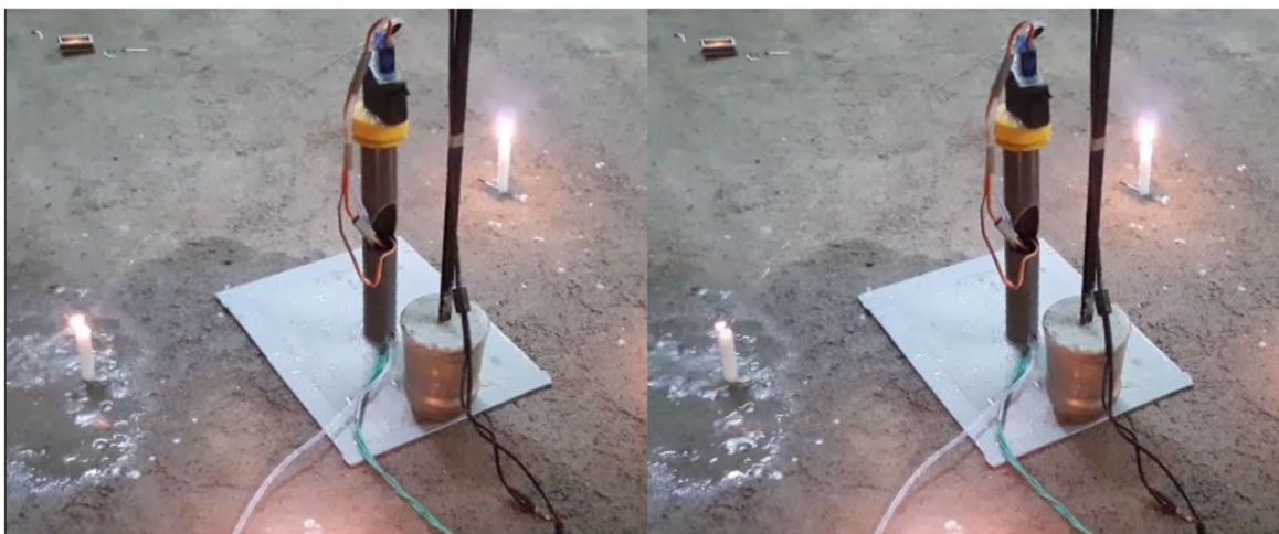
c Jet is hitting the flame but not the wick
