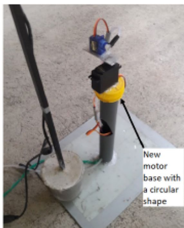
b Revised prototype with circular motor base to enable smooth water hose movement
