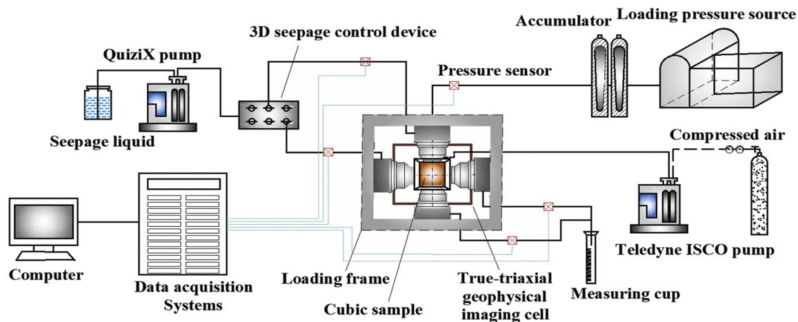
Fig. 6 True triaxial equipment
