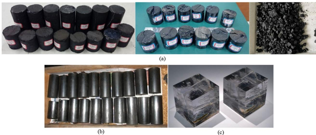
**Fig. 2** Macroscopic comparison of three coal types: **a** Common coal samples (Zhang et al. 2018a, b; Kan et al. 2021), **b** Briquettes, **c** New material coal samples
