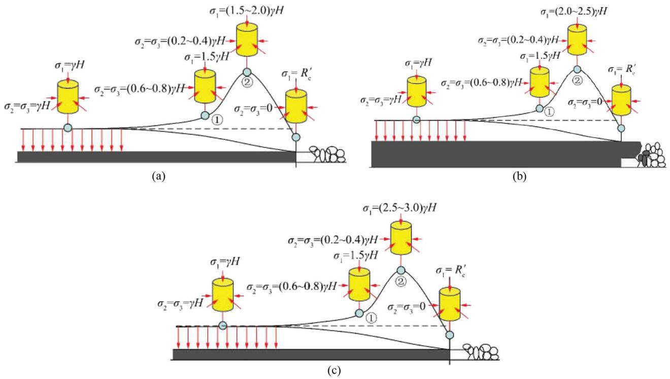
Fig. 4 Three kinds of mining actual stress paths (Xie et al. 2011): **a** Protected coal seam mining, **b** Top-coal caving mining, **c** Non-pillar mining
