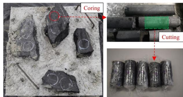
**Fig. 1** Coal samples for uniaxial compression and cyclic fatigue loading
