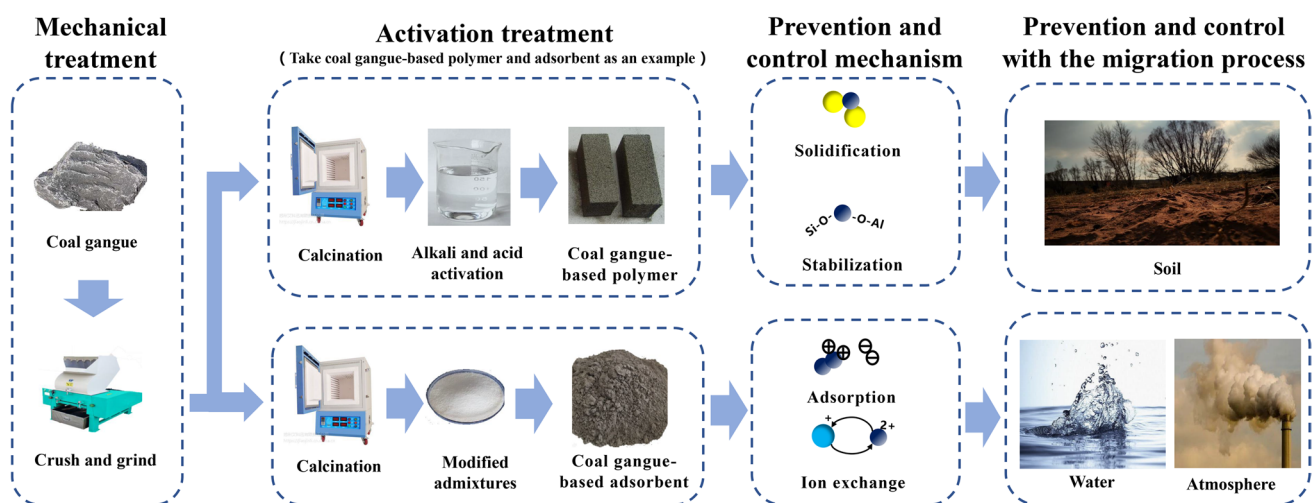
Fig. 4 Prevention and control measures and mechanism of Pb in coal gangue
