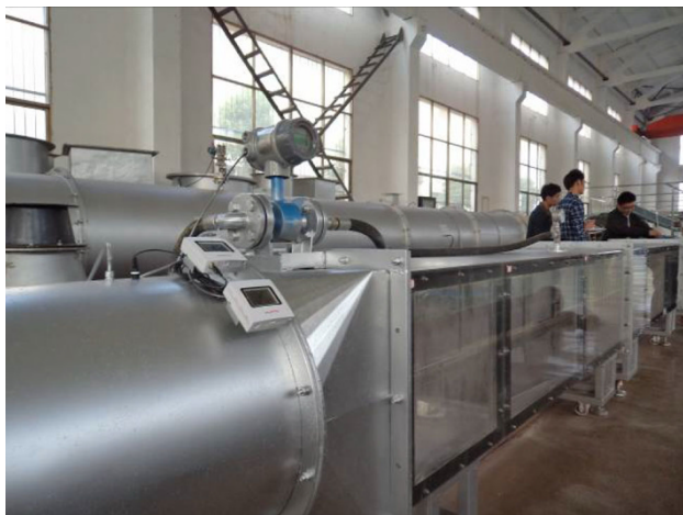
Fig. 8 The photo of a general experiment system of dust removal devices for underground coal mines
