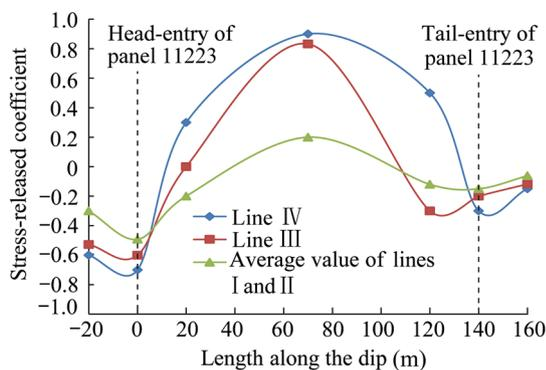
**Fig. 5** Stress-relief coefficient curves in different strata
