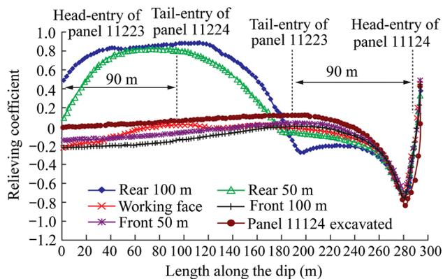
**Fig. 7** Stress-relief coefficient curves in different dip sections
