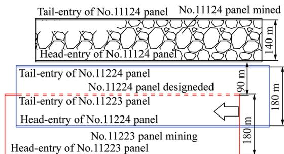
**Fig. 1** Layout of the longwall panels of seams A3 and B4
