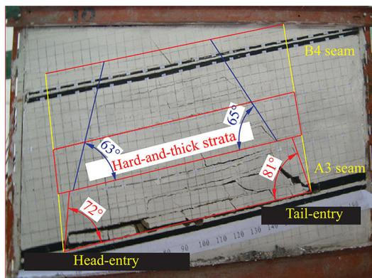
**Fig. 4** Stress-released zone and mining-induced fracture in the coal bearing strata
