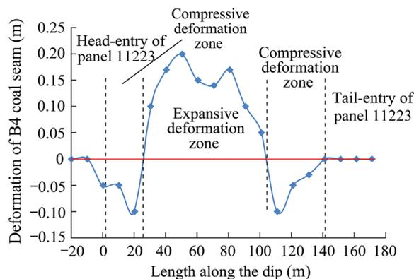
**Fig. 6** Deformation curve of B4 coal seam
