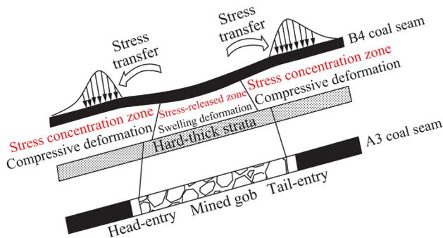
**Fig. 10** Schematic diagram of the stress-relief area in upward relieving mining of hard thick strata
