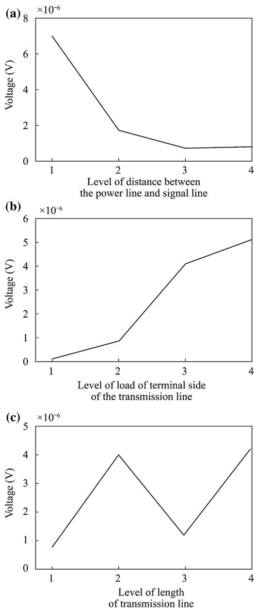
**Fig. 4** Interference voltage of S-terminal for parameters at four levels. **a** Level of distance between the power line and signal line; **b** level of load of terminal side of the transmission line; **c** level of length of transmission line
