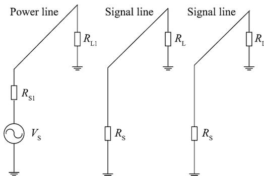
Fig. 2 Model of three parallel conductor transmission lines
