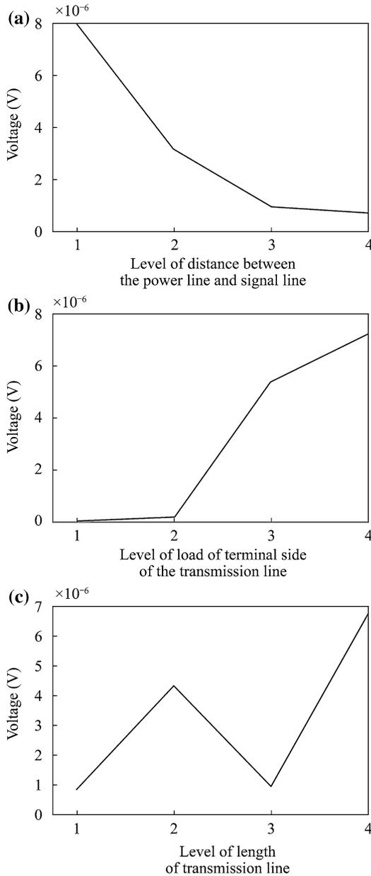
**Fig. 5** Interference voltage of L-terminal for parameters at four levels. **a** level of distance between the power line and signal line; **b** level of load of terminal side of the transmission line; **c** level of length of transmission line
