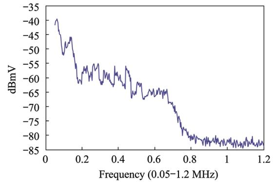
**Fig. 1** The average value envelope spectrum of interferential voltage on device’s power line while working normally
