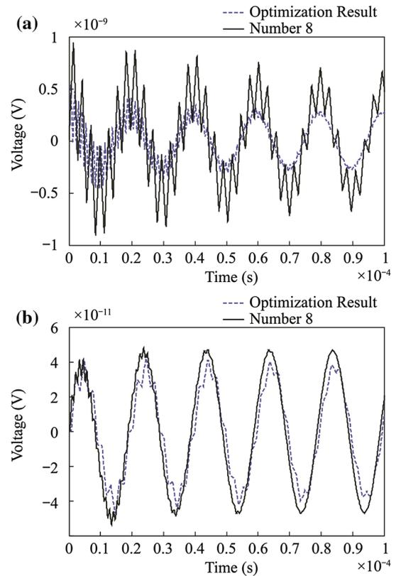
**Fig. 6** Comparison-interference voltage of between optimization result and trial no. 8. **a** interference voltage of S-terminal; **b** interference voltage of L-terminal
