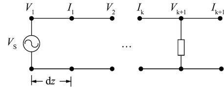
Fig. 3 Spatial discrete of parallel conductors
