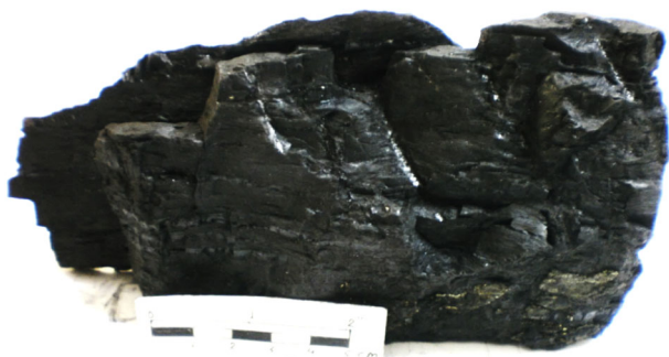
Fig. 1 A cross-section through a lump of coal showing vitrain, clarain, durain and fusain bands with mineral matter
