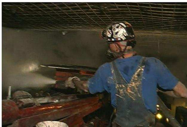
**Fig. 6** Manual application of rock dust in a new face area
