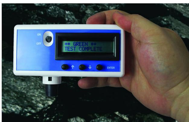
**Fig. 7** NIOSH developed coal dust explosibility meter (CDEM)
