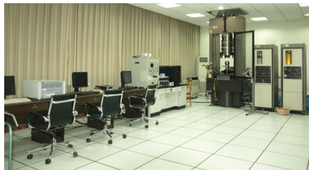
Fig. 1 MTS 815 flex test GT rock mechanics testing system
