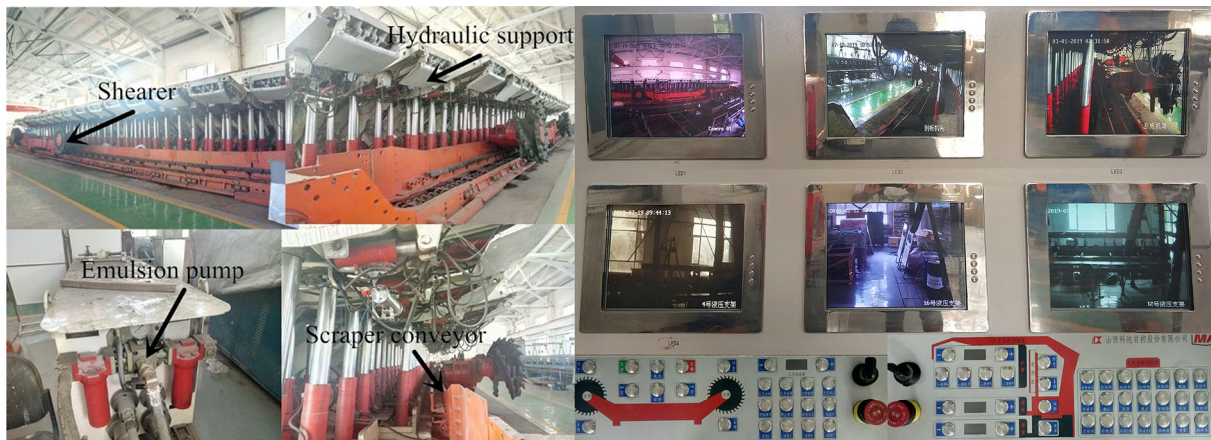
Fig. 9 Three machines experimental platform for fully mechanized mining
