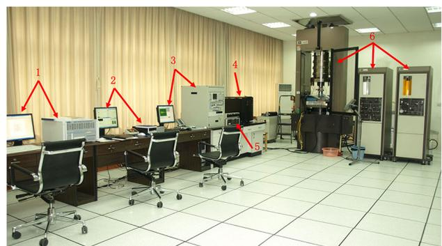
**Fig. 1** MTS815 Rock Test System, which comprises six subsystems: 1—an acoustic three-dimensional positioning and collection system; 2—an MTS815 process control and acquisition system; 3—an ultrasonic excitation and acquisition system; 4—an MTS815 control center; 5—a high-temperature control system; 6—a loading system (axial, seepage, and confining pressures)
