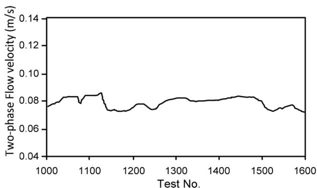
**Fig. 5** Two-phase flow velocity when standard gas output is 2.976 m<sup>3</sup>
