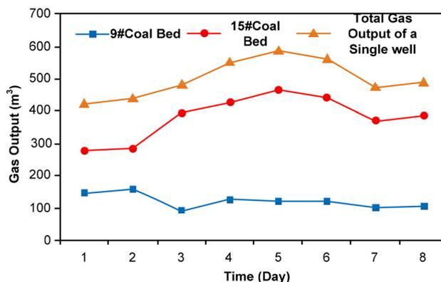
Fig. 9 Gas outputs from different coal seams
