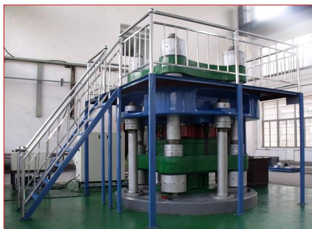
**Fig. 1** Simulation test device to study the fracture mechanism and support technology of surrounding rock in a deep tunnel
