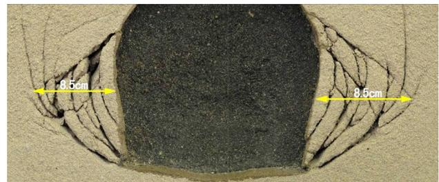
**Fig. 9** Width of cracks in the M2 model
